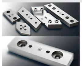
To guarantee the maximum lifetime and best cutting efficiency, scrap metal recycling knives are manufactured only from high-alloyed tool steels. Through-hardening and custom heat treatment ensure optimal hardness, whereas close tolerance ensures a perfect fit.
