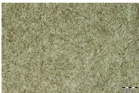
Fig. 7b: Heat treated (Q+T)
