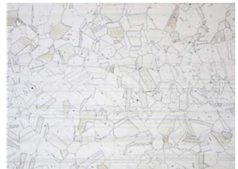
*Figure 1: Austenitic microstructure*
