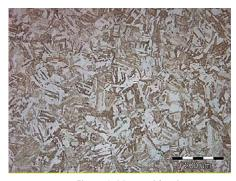
Figure 1: Martensitic microstructure
