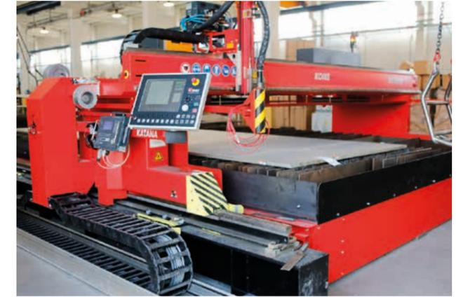
SIJ | Griffon & Romano's latest generation plasma-cutting machinery sets new possibilities to satisfy our customers in the field of stainless steel service. It combines the latest developments in high definition and control technology and provides flexibility of productivity, allowing extraordinary precision cutting for steel plates of large dimensions in heavy-duty production environments.
