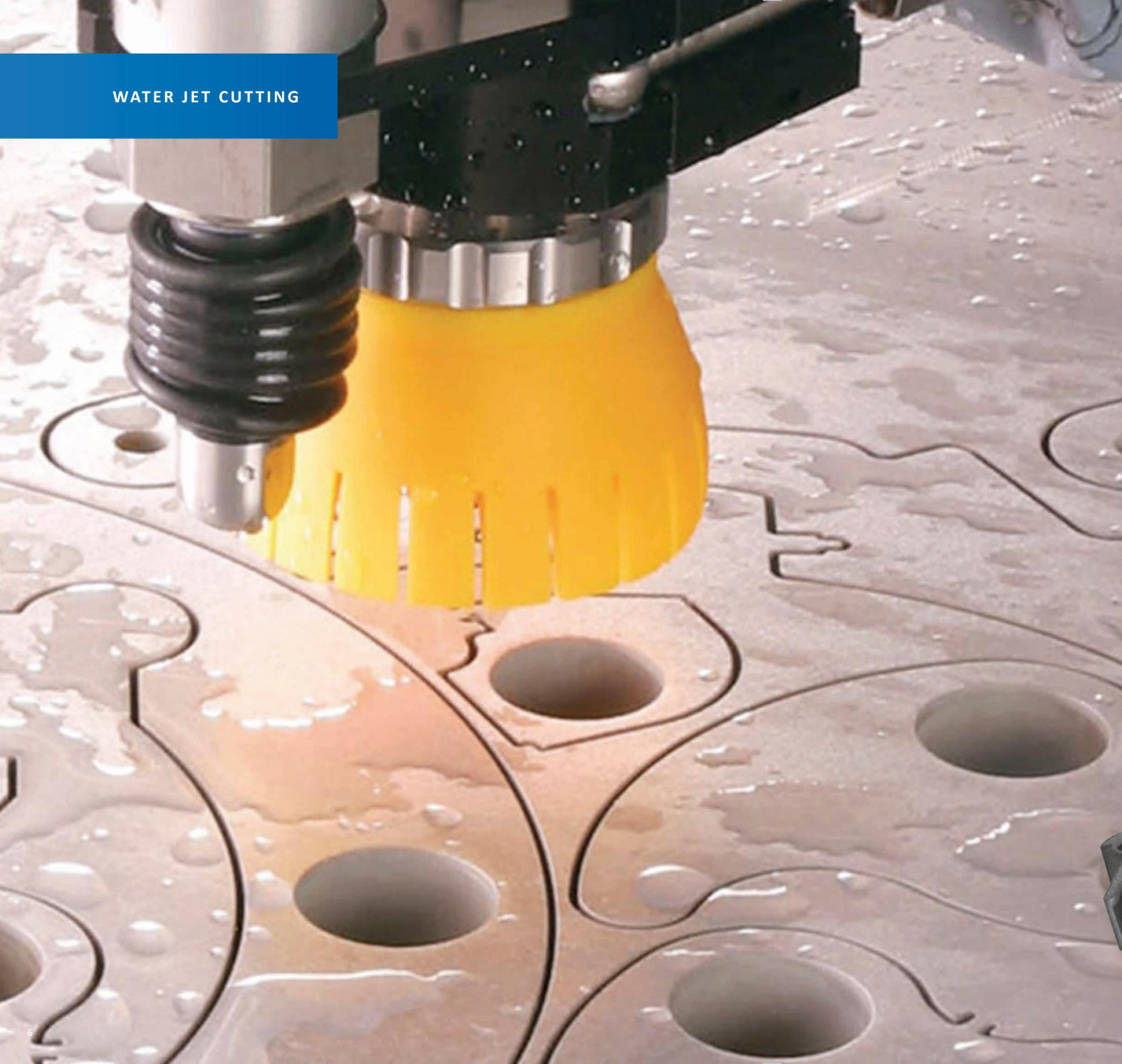
The material is cut by using high-pressure jet of water and abrasives that permit not to alter the chemical-physical characteristics of the material.
